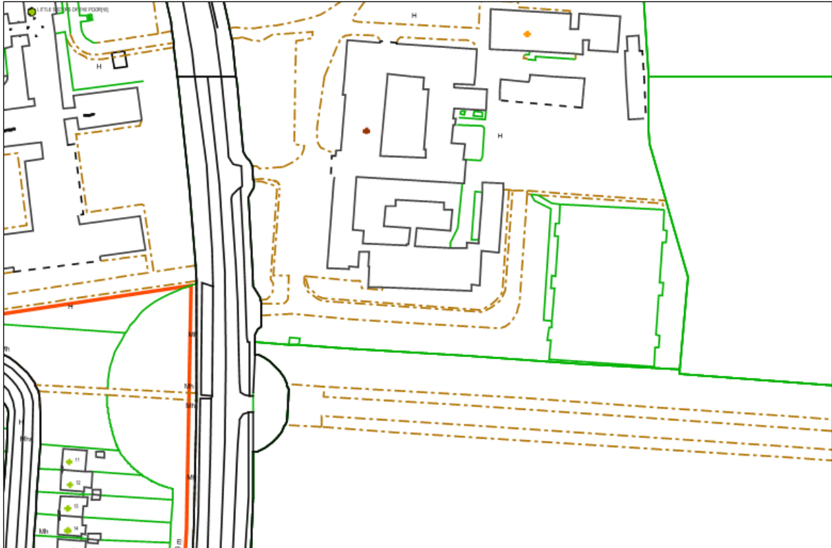
Figure 12-18: Virgin Infrastructure along Sybil Hill Road (Source: Virgin)
